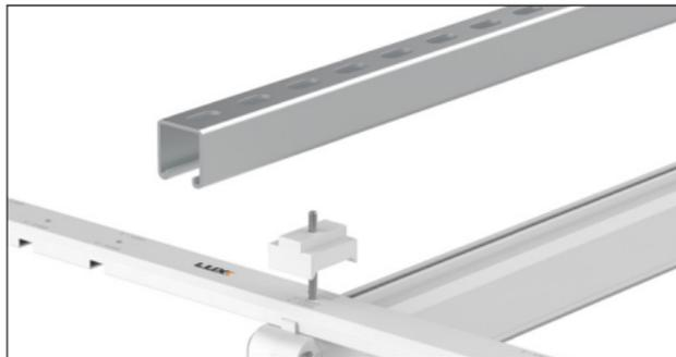
3. Lift the 200w LED Bar, Bar Bracket, hex bolt and Unistrut cleat up through the slot in the Unistrut.
